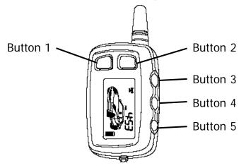
The Astra's 777 2-way LCD remote transmitter is offering increased range and confirmation of any activated feature.
